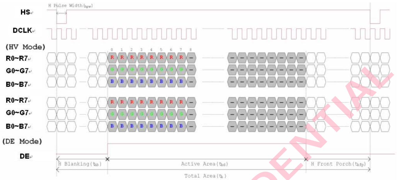
Figure 3. 1 Horizontal input timing diagram.
